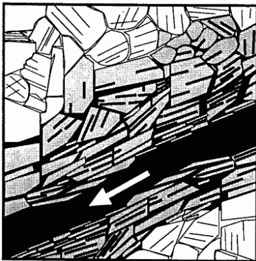
Fig. 28: Flow in a fracture
