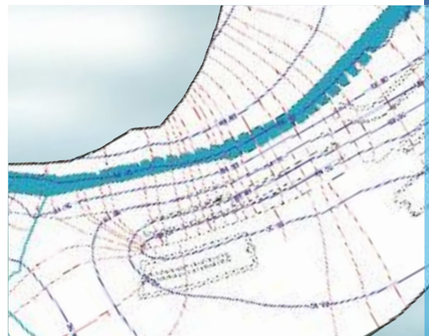
Precise predictions: Calculation of flow lines for delimiting and representing catchment areas and determining travel times.
